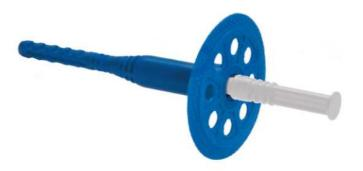
Used for the mechanical anchoring of insulanting panels, mineral wool and for all main types of masonry, for the purpose of sustaining the load and tensile stress. The preassembled nail significantly facilitates and speeds up the application of the plugs, allowing the user to save time during installations.
